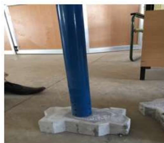
Fig4.4 Impact test on paver block
