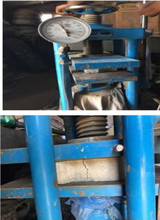
Fig 4.1 compression testing on paver block
